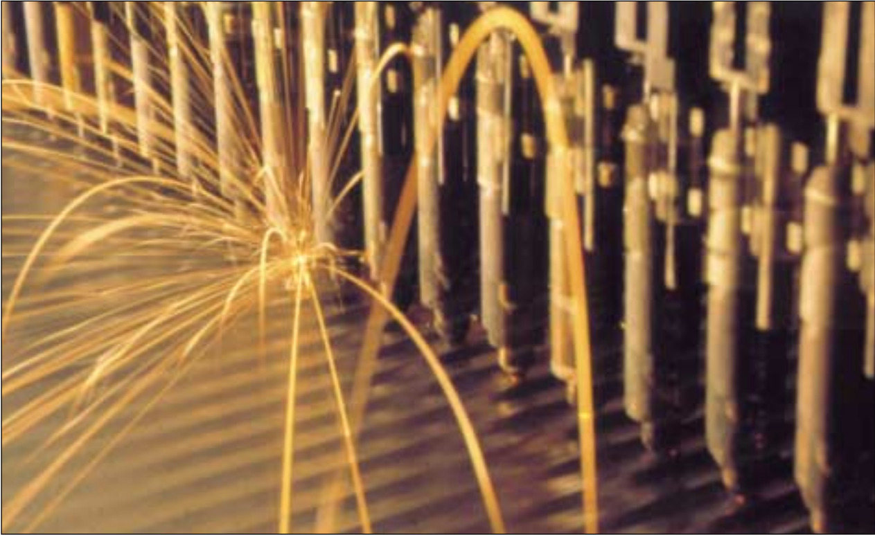
"Solahart use fully automated processes for manufacturing absorber panels"
