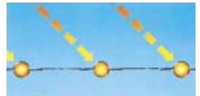
Standard fin and tube style absorber panel.
